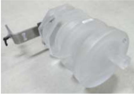
Gambar Water phantom CT Scan
